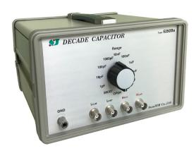
Type 6250B is a decade capacitor whose value can be set as 1 pF to  $100\mu$ F for 4-terminal measurement. Type 6250B can be used as a standard for calibrating LCR meters as its excellent accuracy and stability.
