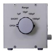
VAC Series are 4-Termianl Capacitance Standards. Ten built-in capacitances and dissipation factors between 1pF and 1µF can be selected within the specifications shown below. OPEN·SHORT range is equipped as standard, correction can be made with cables connected. VAC Series can be used as a standard to calibrate LCR Meters as stability is excellent.
