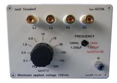
6270A Series are highly stable tan  $\delta$  (Dissipation Factor) standards which are made of ceramic capacitance and accurate resistor. tan $\delta$  (Dissipation Factor) calibration can be made at 120Hz and 1kHz by switching.
