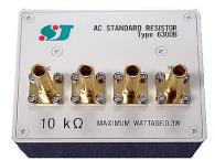
6300B was designed under the technical guidance of NMIJ/AIST (The National Metrology Institute of Japan/The National Institute of Advanced Industrial Science and Technology/). The precision AC standard resistor realized AC-DC error less than 10 ppm at under 10 kHz and phase angle error less than 50µrad. The resistance is extremely stable thus it can be used as a resistance standard for DC as well as AC.
