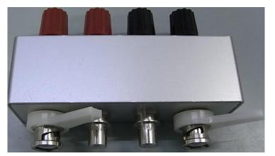
Convert connector of 4-terminal BNC type LCR meter to binding post
