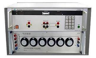
Model 1010A is a power calibrator which compares a target power meter with a calibrated power meter. The system consists of a Current Transformer and a Voltage Transformer. It can calibrate power meters, for example, comparing a target power meter in the range of 0.05mW to 666.666W with a reference power meter calibrated at 100 V, 5 A.
